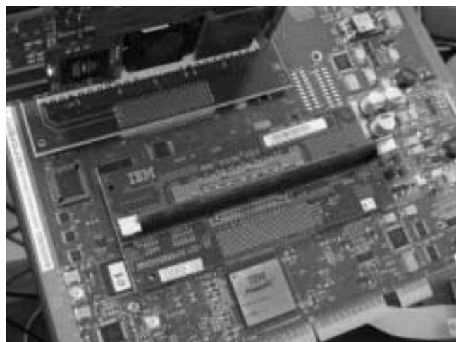
Figure 6: Board used for debug with DDR2 DIMMS close to the IOP processor and PCI-X bus analyzer
